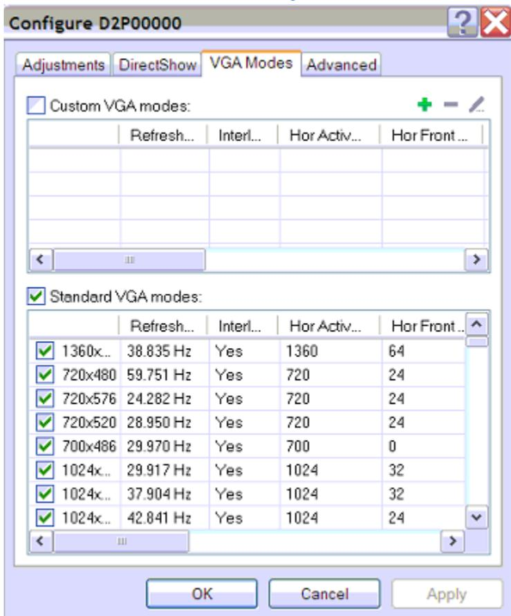
Use this tab to select the standard VGA modes that are used during image capturing. The **Standard VGA modes** checkbox allows you to select all standard modes. To apply several modes select the checkboxes near the mode resolution value.
